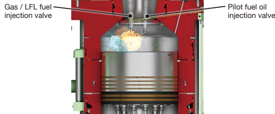
Combustion chamber for ME-GI/LGI
