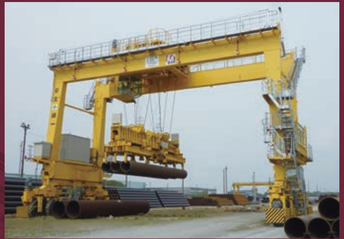
Rubber-Tyred Pipe Handling Crane
