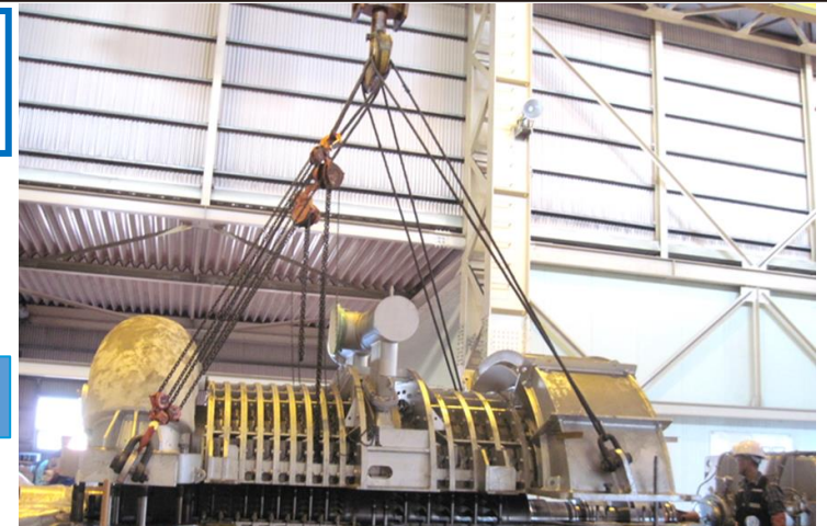
One point lifting up upper casing for easy overhaul and internal inspection
