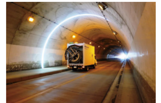
Tunnel Lining Scanning Car "Tunnel Catcher 3"
