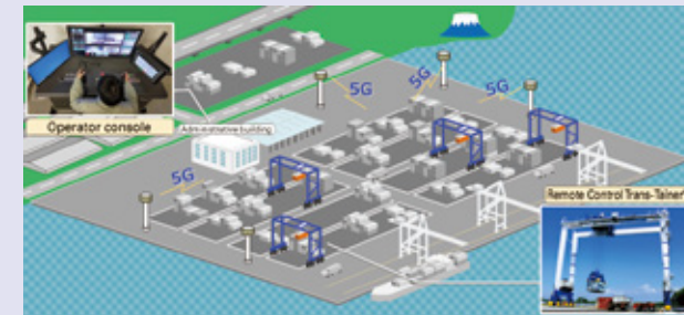
Diagram of the local 5G communication equipment configuration at the container terminal
