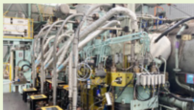
Hydrogen combustion test on our test engine
