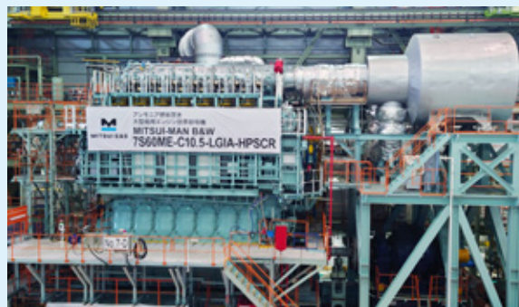
The world's first commercial Large-bore Two-Stroke Low-speed ammonia dual fuel engine
