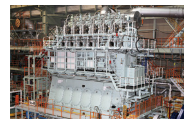
Electronically-controlled gas injection diesel engine 「ME-GI」
