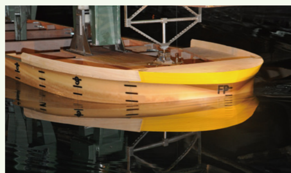
Water tank tests using a model at Akishima Laboratories (Mitsui Zosen) Inc.
