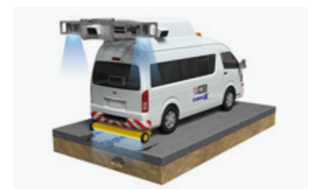
Vehicle for radar inspection
