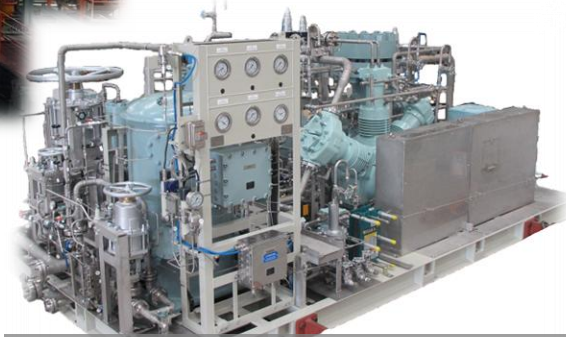
High Pressure BOG Compressor
