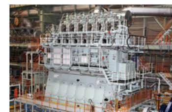
Electronically-controlled gas injection diesel engine 「ME-GI」
