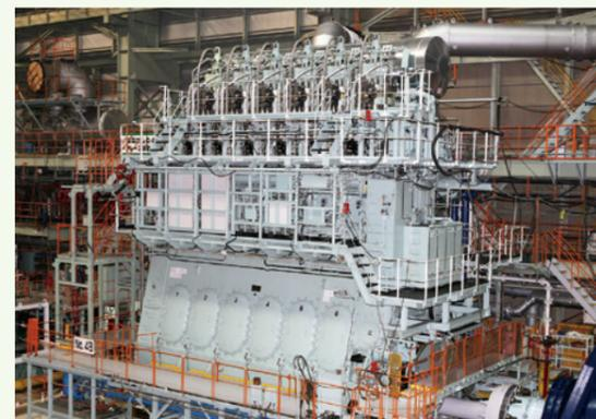
Electronically-controlled gas injection diesel engine (ME-GI)
